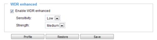
Note that the **Preview** button has been cancelled, all changes made to image settings is directly shown on screen. You can click **Restore** to recall the original settings without incorporating the changes. When completed with the settings on this page, click **Save** to enable the setting. You can also click on **Profile** to adjust all settings above in a pop-up window.
